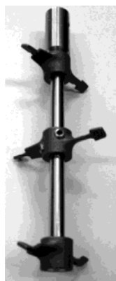
Figure 2. (a) Three-stage Ekato MIG. (b) Two-stage turbine.
